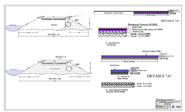
Figure 3.6: X-Section of the Road Restoration Works
