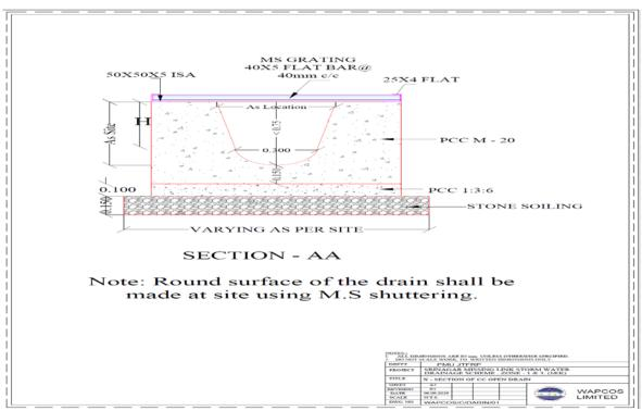
Fig 3.3: Cement Concrete Drainage Section
